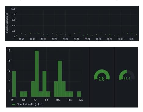
The final figure shows the spectral width for the direct connection, via a shielded precision attenuator system, of the ZachTek WSPR-TX XP Plus transmitter with a 10 MHz Bodnar external reference source and the RX888 MKII receiver using a 26 MHz external Bodnar reference source. This figure shows the spectral width vs. time, and all of the values are 11 mHz.
