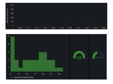
The following two figures show the spectral width for the direct connection of the ZachTek WSPR-TX XP Plus transmitter with its 25 MHz internal reference source and the RX888 MKII receiver using a 26 MHz external Bodnar reference source. This first figure shows the spectral width vs. time and the second figure shows a histogram of the spectral width samples.
