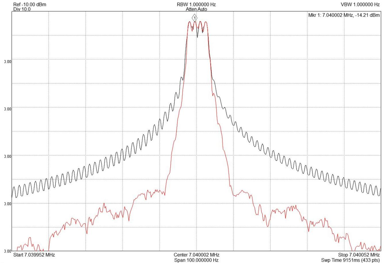
WSPR FSK and FST4W-120 GFSK spectra
