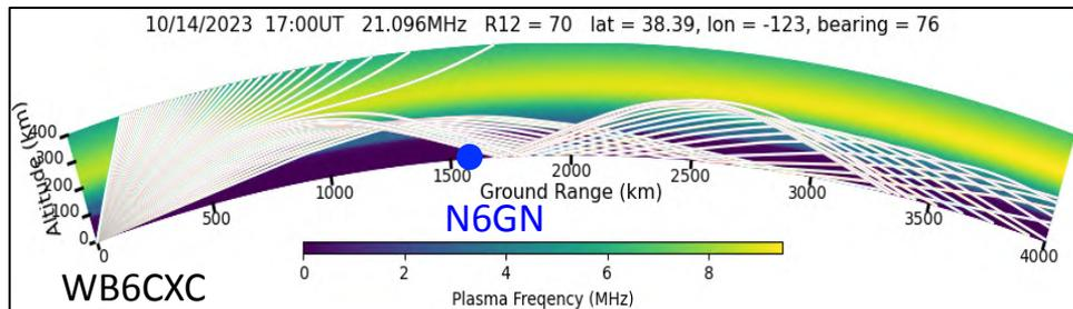
**15 m** Consistent picture: One-hop when unaffected by eclipse, and within skip zone if sunspot number dropped to 70, as for the TI4JWC-ND7M path.
