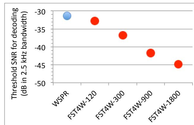
Defined at 50% probability of decode with Doppler spread of no more than 0.01 Hz
