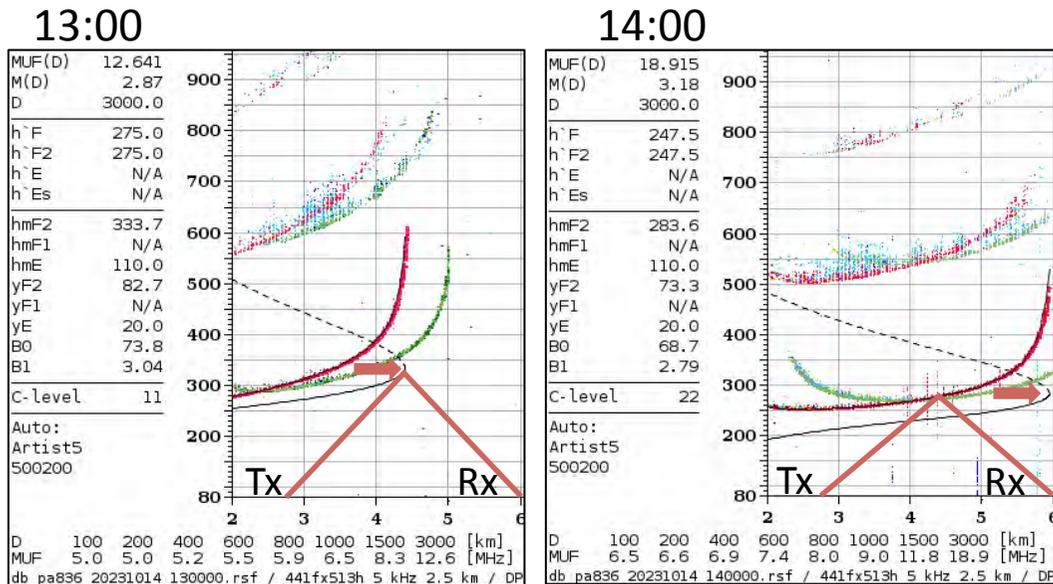
**Why?** To measure the changes in height at which signals refract in the ionosphere as a response to the eclipse.
