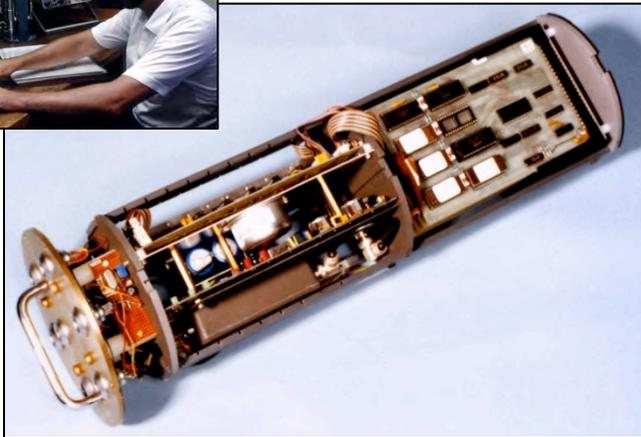
Battery powered (3 months), self-contained Doppler Sonar, 1987. Direct conversion 1 MHz receiver, in-phase and quadrature outputs. RCA CDP1802 CPU, 12 bit ADC and hardware multipliers for frequency analysis.
