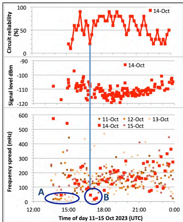
**How can we see this happening?** FST4W and its frequency spread measurement.
