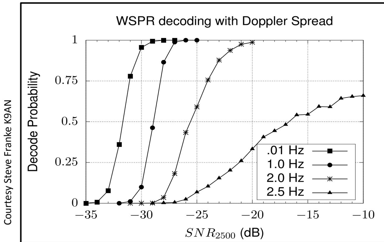
Here, 'Doppler spread' is the span between upper and lower -10 dB points of the signal's spectrum.
