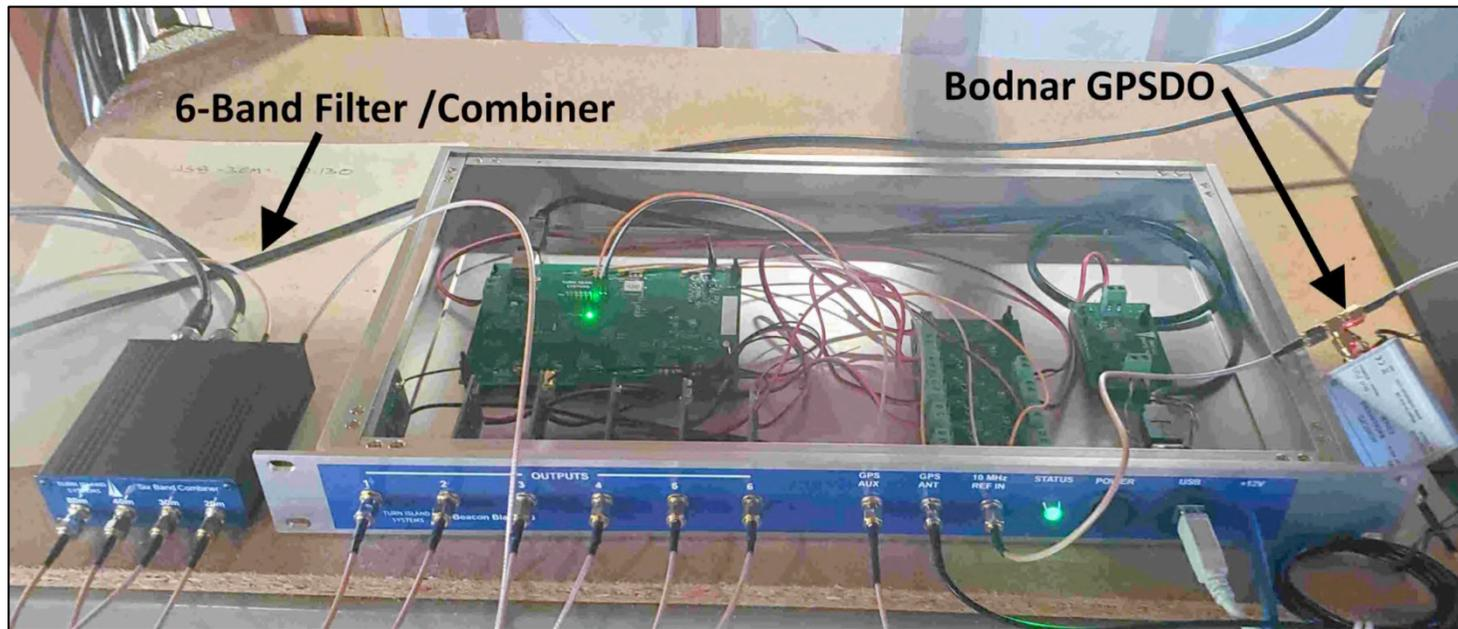
Designed specifically for FST4W operation during the October 2023 eclipse the WSPRSONDE-6 from Turn Island Systems can transmit on six HF bands simultaneously with 100% duty cycle. <https://turnislandsystems.com>
