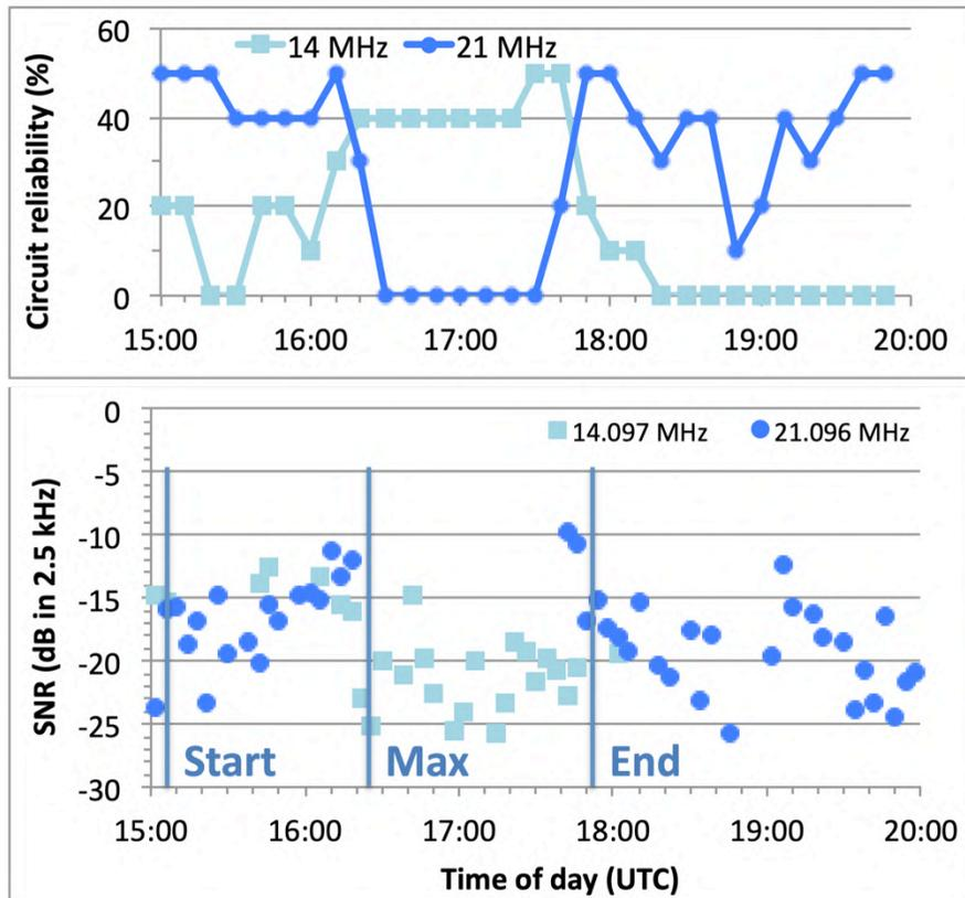
*Circuit reliability (top) and SNR (bottom) at N6GN, N. Colorado for FST4W transmissions from WB6CXC, N. California on 20 m and 15 m.*
