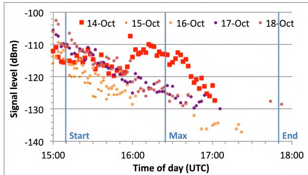
*Signal levels on 14-18 October 2023 at KA7OEI-1, Northern Utah for FST4W transmissions from WO7I, Nevada on 3.57 MHz.*
