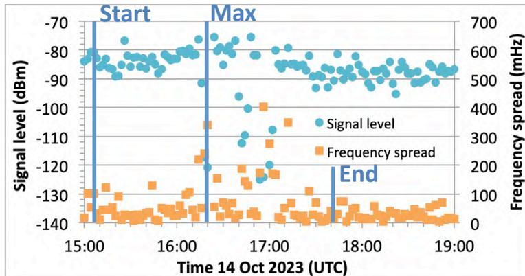
How can we see this happening? FST4W and its frequency spread measurement.
