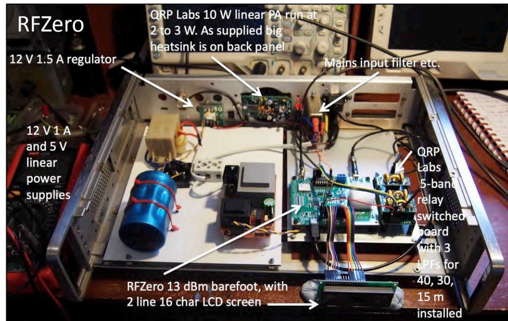
If at all possible use equipment with GPS-aided, or even better, phase-locked GPS disciplined Master Oscillator or an OCXO.
