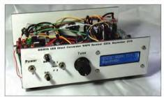
The author's latest version in development. This uses the main heard as described in the article plus an Arduino clone with a ORP Labs Arduino shield and a ORP Labs Si5351A synth for the local oscillator. It covers up to five bands with a ORP Labs relay switched board with the author's own size compatible plug-in single-crystal filters.
