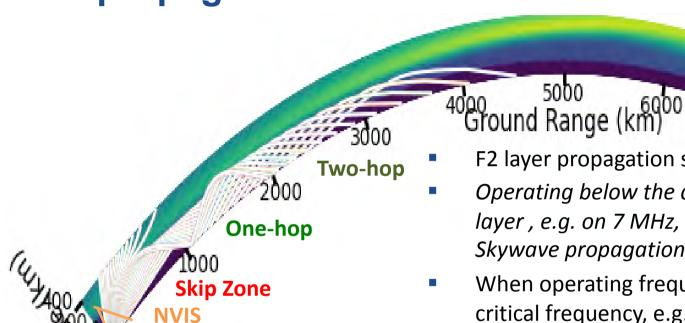
Ray tracing using PyLap
