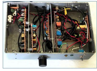
Construction on strip board in a die-cast box. May 2015.
