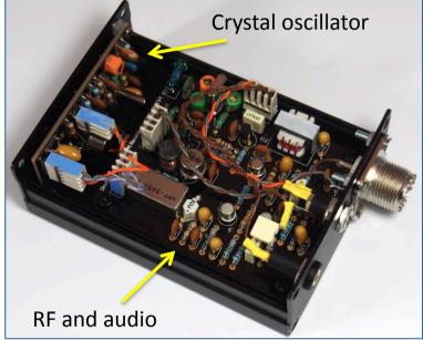
'2016 model'. W3PM design plus David Norton's "noiseless feedback' RF pre-amp and modified crystal oscillator on two PCBs.
